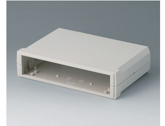
B3020117 MOTEC M, flat/flat ABS (UL 94 HB) off-white RAL 9002 205x140x50mm IP 40
