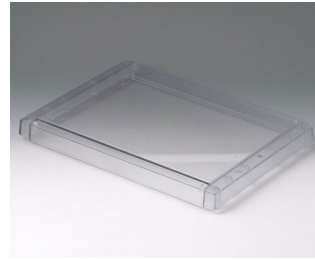
B4030621 Cover L, flat PC (UL 94 V-0) transparent 302x220x29mm
