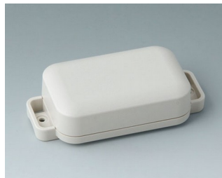
C3204207 EASYTEC 80 ASA+PC (UL 94 V-0) off-white RAL 9002 101x50x26mm IP 65 opt., IP 40
