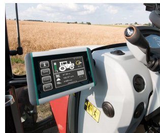
ISOBUS terminal for tractors and self-propelled machines
