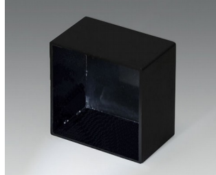
A8032208 POTTING BOXES, Vers. III PA 66 (UL 94 V-2) black RAL 9005 32.4x32.4x20mm
