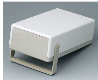
A9040165 FLAT-PACK CASES 189 N, Vers. II ABS (UL 94 HB) off-white RAL 9002 189x110x60mm IP 40
