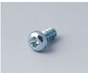
A0305031 Self-tapping screws 2.5 x 6 mm (PZ1)
