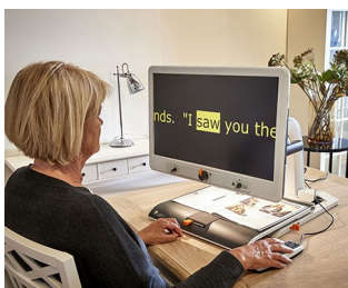
Control knobs for video magnifier
