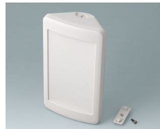
B4610207 SMART-CONTROL M, Vers. II ASA+PC (UL 94 V-0) off-white RAL 9002 173x101x59mm IP 40, IP 55 opt.
