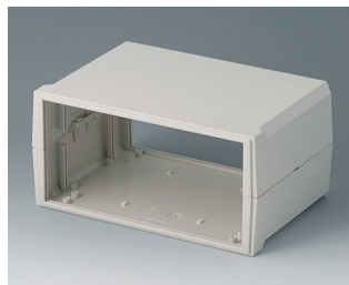
B3020137 MOTEC M, high/high ABS (UL 94 HB) off-white RAL 9002 205x140x100mm IP 40
