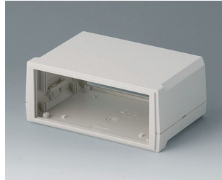
B3015127 MOTEC S, flat/high ABS (UL 94 HB) off-white RAL 9002 155x105x65mm IP 40
