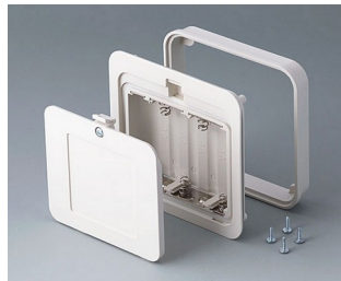
A9338117 Battery compartment kit, 5 x AA ABS (UL 94 HB) off-white RAL 9002 93x98mm IP 54
