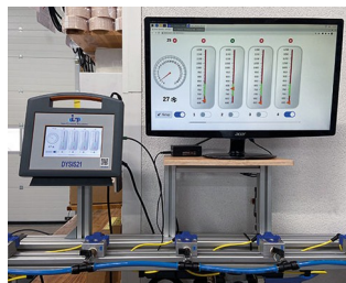
Monitoring system for cleaning nozzles
