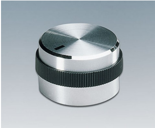
A1421469 TUNING KNOB, with lateral screw fixing ABS (UL 94 HB) brilliant 22.1x14.3mm 6mm
